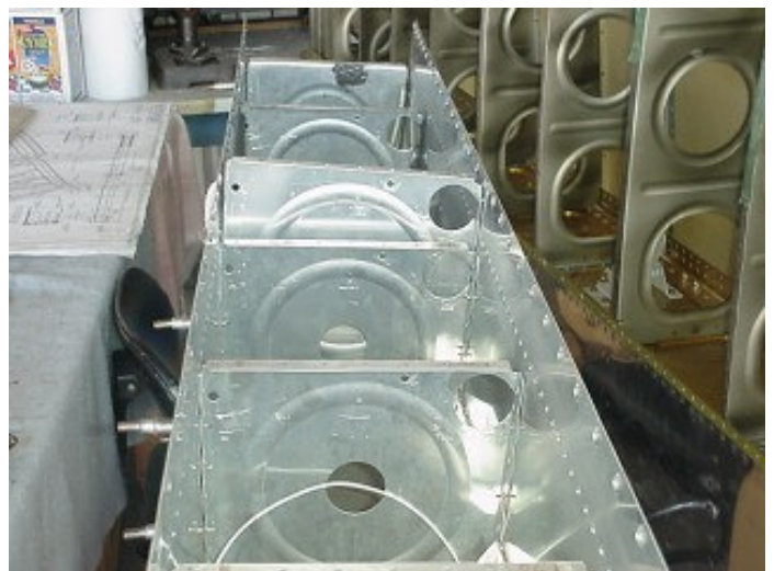
Bob Raines begins the messy task of sealing the fuel tank on his RV-7A.
